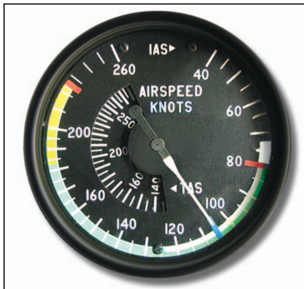
Figure 12-1. Airspeed indicator markings for a multiengine airplane.
